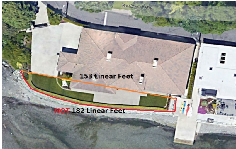
Figure 23: Determination of Length of Shoreline Stabilization. Google, 2022, Landsat / Copernicus - modified with polygons and text.
